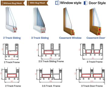
· Multi -chamber profile design, frame depth from 52 to 112 mm
